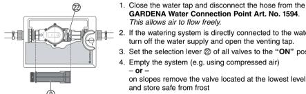
Valves can be easily removed from the box.
